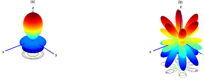
Figure 7-4: Angular plots of \text{Re}(\Theta(\theta)\Phi(\phi)) evaluated for a 8.6863 Debye dipole at the origin. The negative z -axis corresponds to the position of a negative partial charge. Figure 7-4 (a) depicts a 4s\sigma orbital which is strongly polarized away from the negative charge, and (b) depicts a 4f\phi orbital which resembles a hydrogenic orbital.
